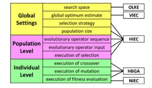
Fig. 3. Levels of search control granted to the user by online knowledge embedding (OLKE), visualized IEC (VIEC), HIEC, HBGA, and NIEC. As shown in this figure, these technologies are not mutually exclusive and can therefore complement each other.
