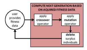
Fig. 1. Control flow of a narrowly defined IEC (NIEC) application. The user is prompted for fitness information once each generation but has no control over the overall search dynamics.
